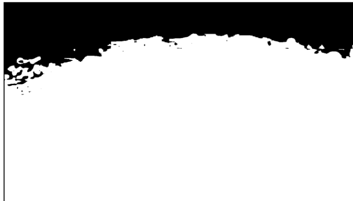
Fig. 2c. Silhouette of scale on carburized layer (950°C for 2 hrs, X200) (Dark upper region represents enhanced hardened case)
