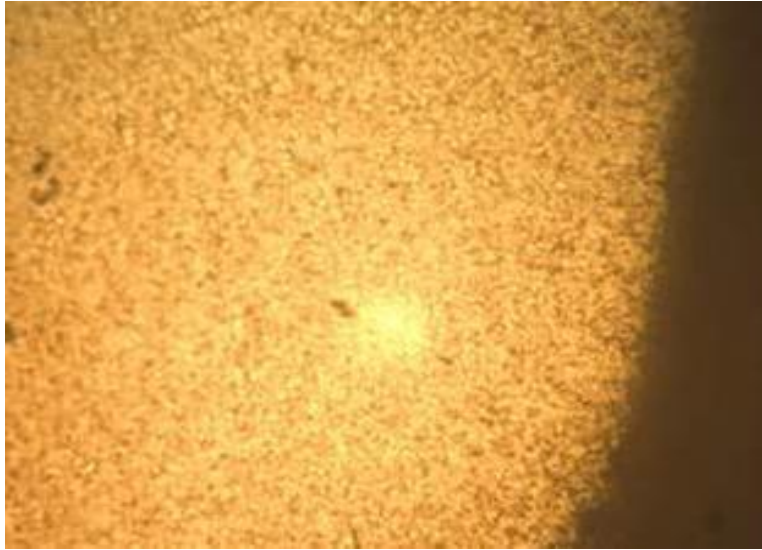
Fig. 11. Sample treated at 550°C for 2 hrs, X100
