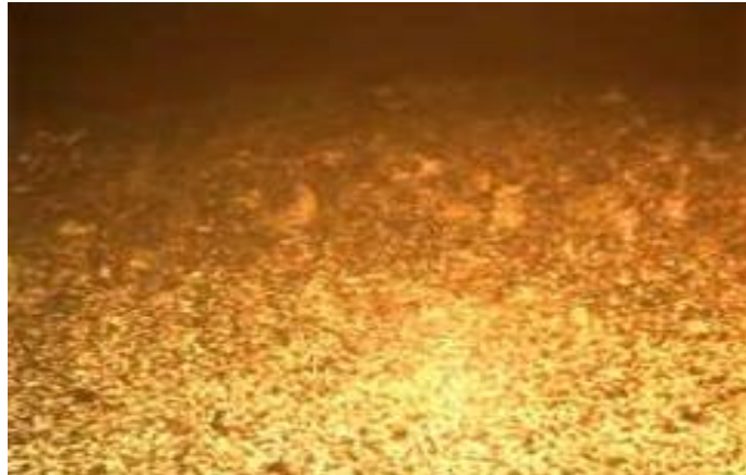
Fig. 2a. Sample treated at 950°C for 2 hrs, X200 (Dark upper region represents case)
