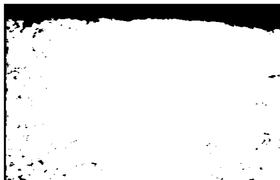
Fig. 4c. Silhouette of scale on carburized layer (950°C for 4 hrs, X200) (Dark upper region represents enhanced hardened case)
