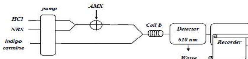
Fig. 4. Schematic diagram of the FIA-spectrophotometric manifold used for the determination of AMX
