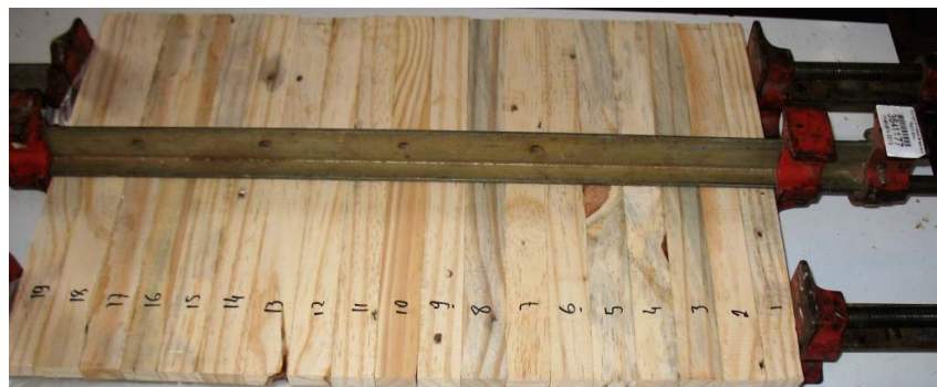
Fig. 2. Pressing procedure of the core battens
