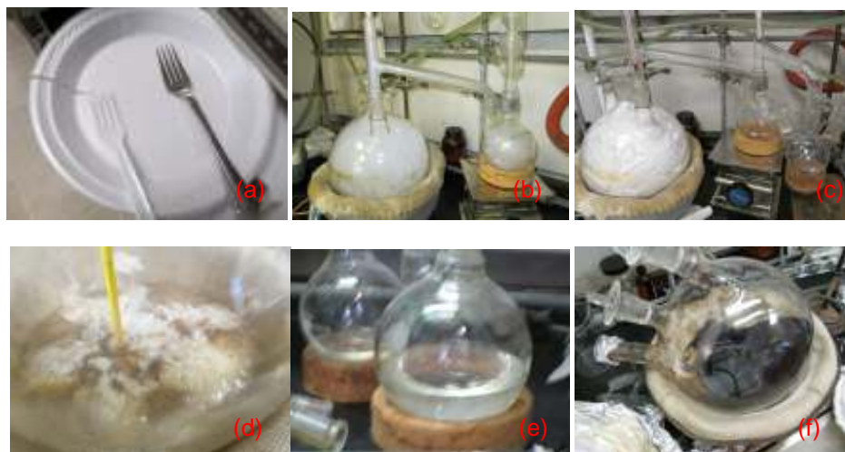
Figure 1. Step-by-step illustration of decomposition process of SDP: (a) SDP and utensils; (b) the reactor loaded with the first load of shredded SDP; (c) reactor charged with the second load of SDP; (d) inserted thermometer into melted SDP; (e) condensed liquid; and (f) end leftover
