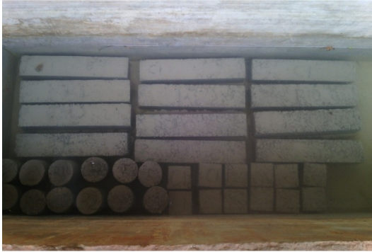
Fig. 2. Samples of specimens water cured
