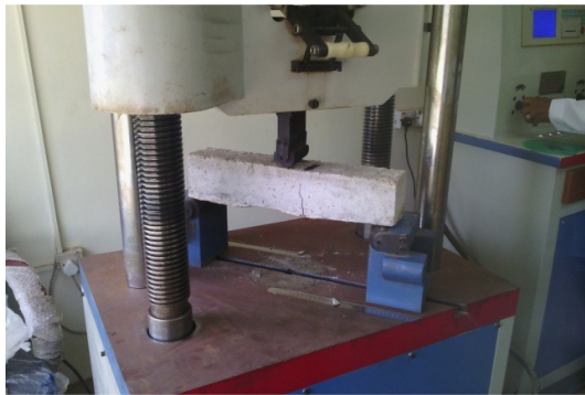
Fig. 3. Specimens undergoing flexural test
