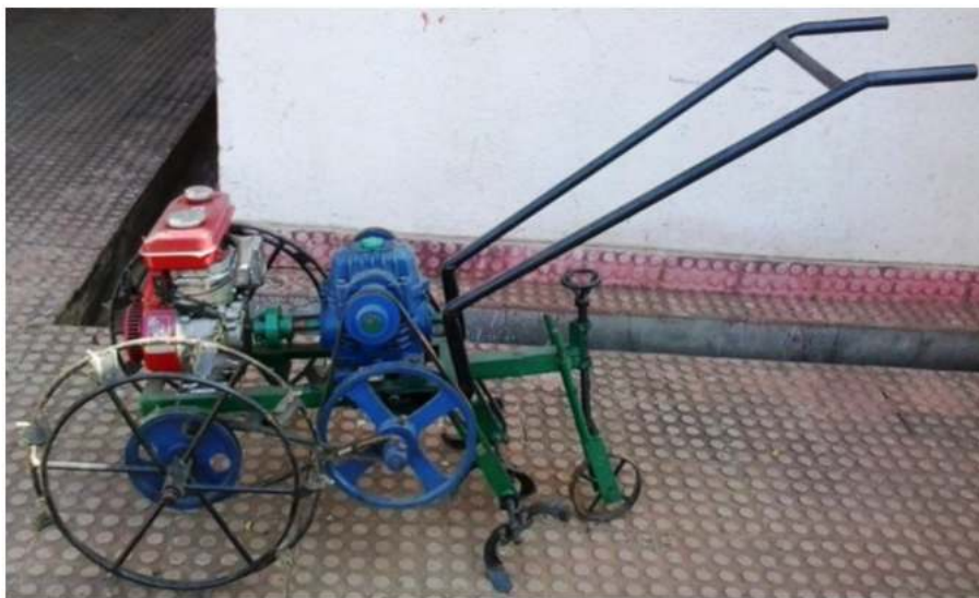
Fig. 2. Developed rotary weeder
