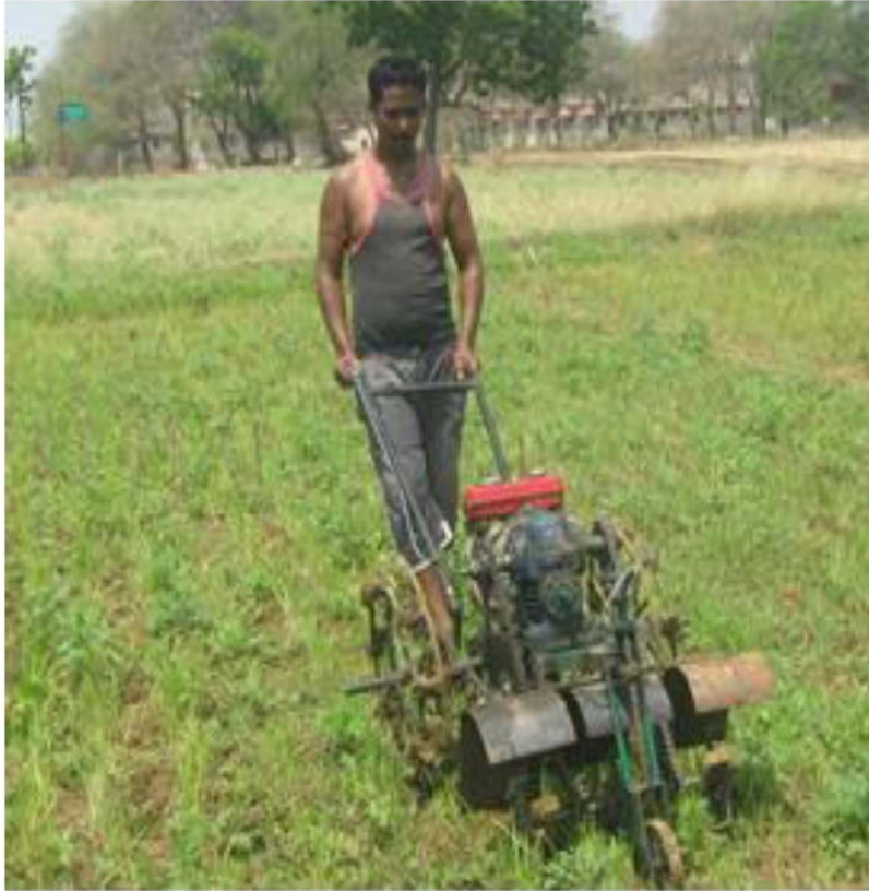
Fig. 3. Developed rotary weeder during field operation
