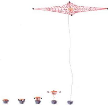
Fig. 4(a). Schematic of net capturing method [19]
