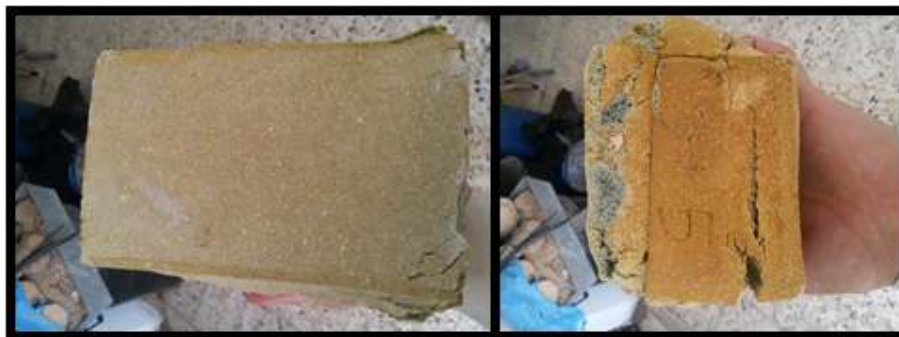
Fig. 5. Negative firing shrinkage fired clay brick with 40% waste glass and firing at 1100°C
