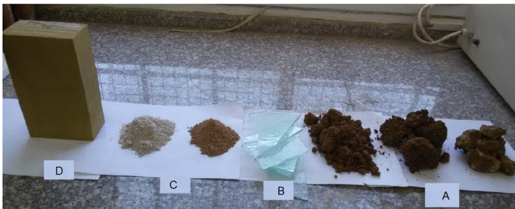
Fig. 4. A) Clay, B) Waste glass, C) Clay and Waste glass powdered, D) Fired clay brick
