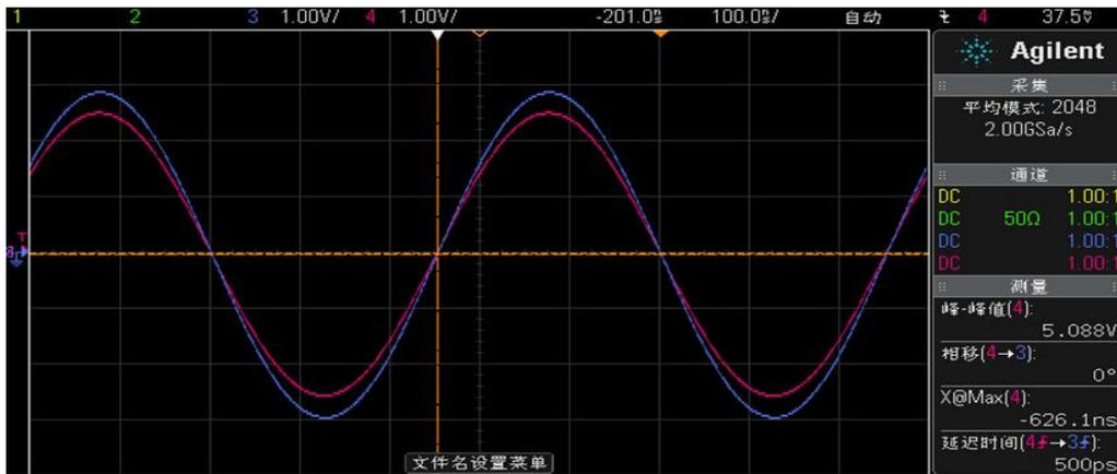
Fig. 3. Display of time delay, 9.4 m versus 0.4 m, at 2.0 MHz
