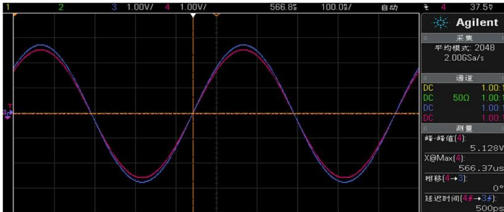
Fig. 2. Display of time delay, 6.4 m versus 0.4 m, at 2.0 MHz
